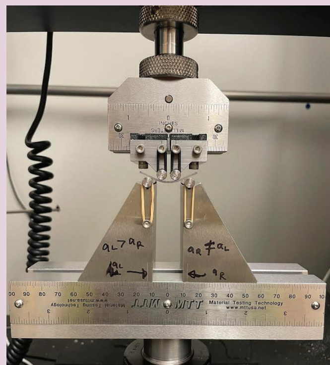
Strength test: ADA Science & Research Institute staff use a four-point bend apparatus to test the flexural strength and modulus, or stiffness, of materials used to produce orthodontic sequential aligners.
